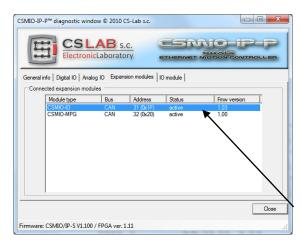
CAN address seen by the CSMIO/IP controller is a number set on module +16 configuration jumpers.
